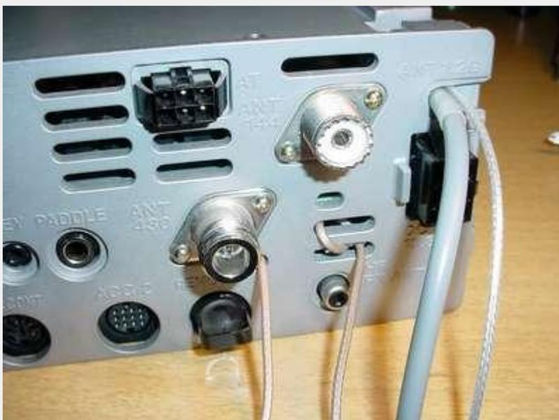
Here is a picture of the back of the modified TS-2000X, showing the three new coaxial inputs.
